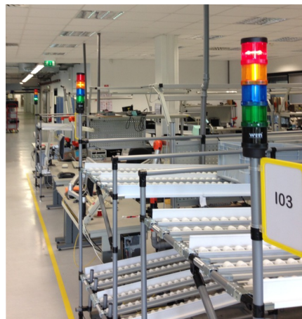
WERMA signal towers and the WIN system are used for material flow and visualisation of the work process.
