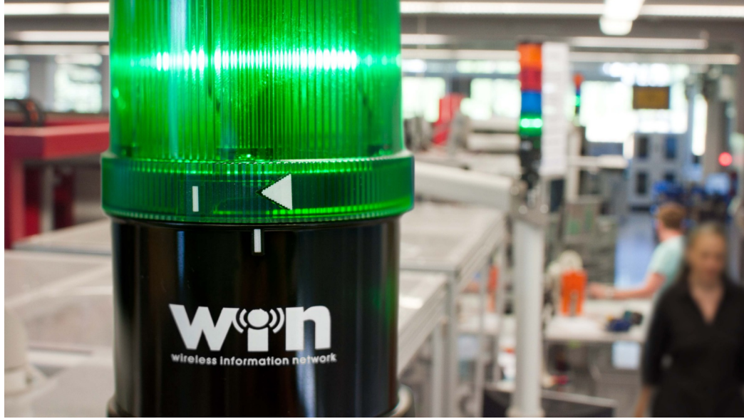
Material flow information transmitted wirelessly allowing stores to replenish required material and deliver on a “first in first out” principal.
