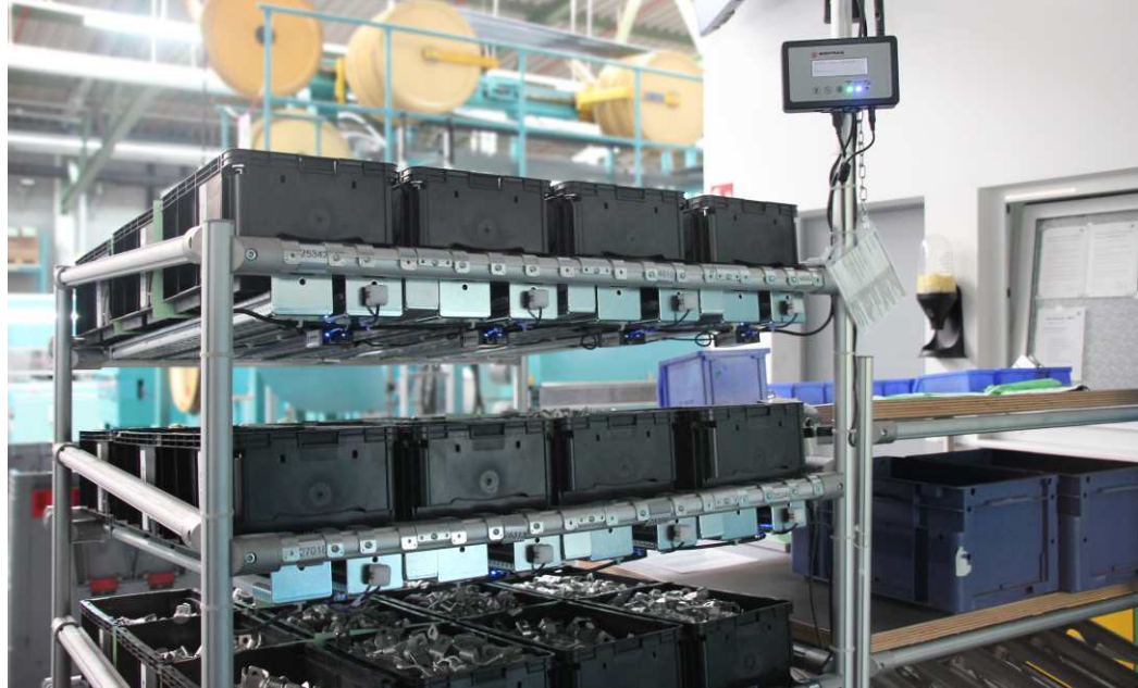
StockSAVER gives complete transparency of stock levels held in FIFO flow racks at Auto-Kabel ensuring that stock does not runout whilst traditional levels of safety stock are reduced.
